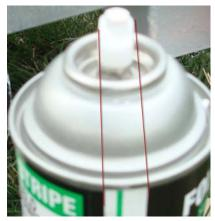
• Once you have the nozzle aligned with the line on the side of the can, now just put the can in the sprayer so the line is perpendicular to front of the sprayer as shown below:
